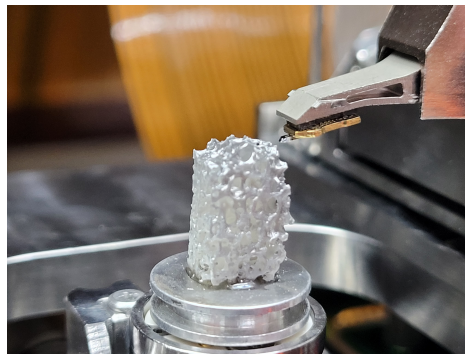
Figure 1: Bone sample mounted inside the FusionScope trunnion stage with the AFM cantilever positioned on top of the sample.
