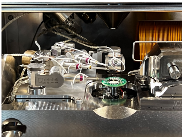
Figure 1: Integration of four Kleindiek micromanipulators inside the FusionScope system. The micromanipulators are fixed on the trunnion allowing for 80° tilt of the whole setup and simultaneous operation with SEM, AFM, and EDS.
